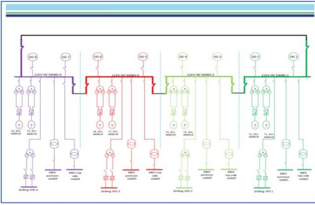
Figure 1 Ring Bus vessel configuration. Image reproduced from DNV GL
